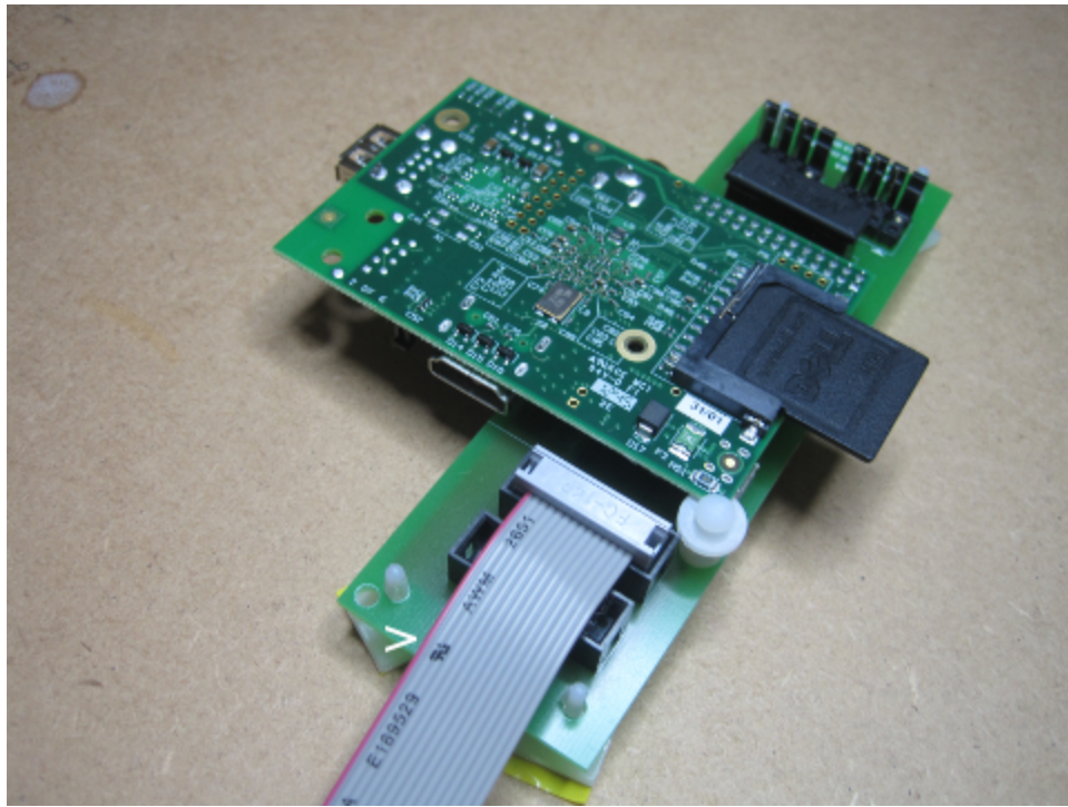
Figure 10 – Pinball DMD Screen ribbon cable – red wire on the left marked with arrow
