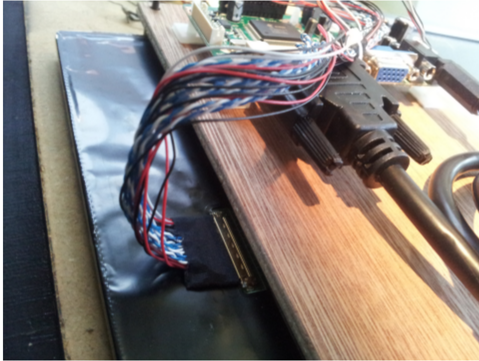
Figure 6 – LVDS cable connected to the LCD screen
