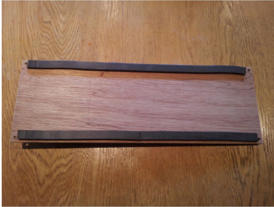
Figure 2 – Foam weather strip on the back of the plywood mounting plate
