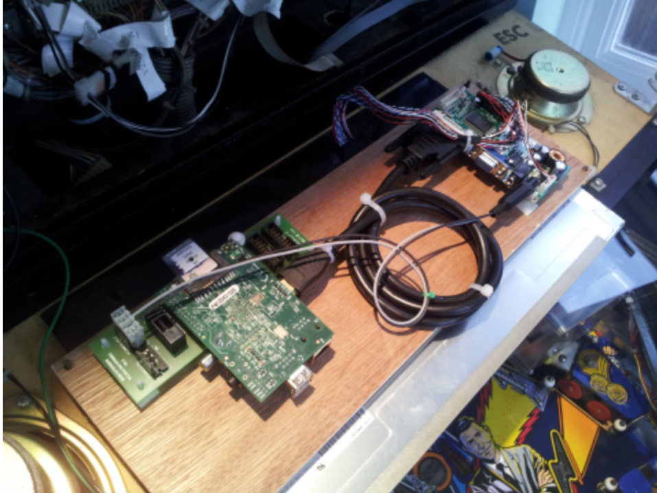
Figure 6 – Plywood mounting panel in place
