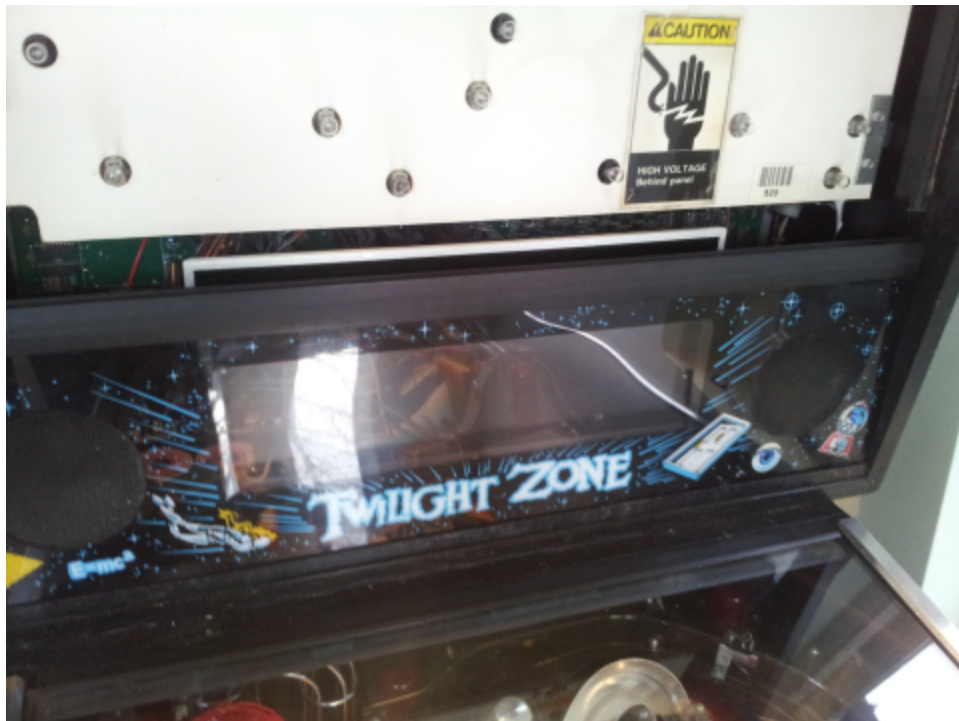
Figure 9 – Check the screen is square to the top of the speaker panel
