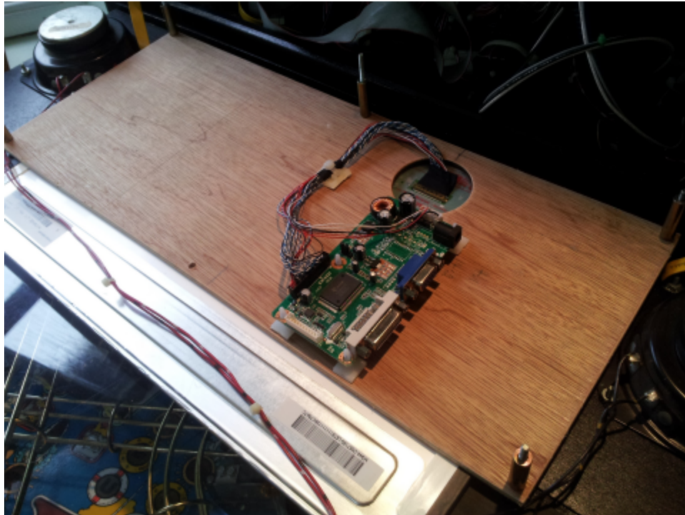
Figure 16 – Plywood mounting panel in place
