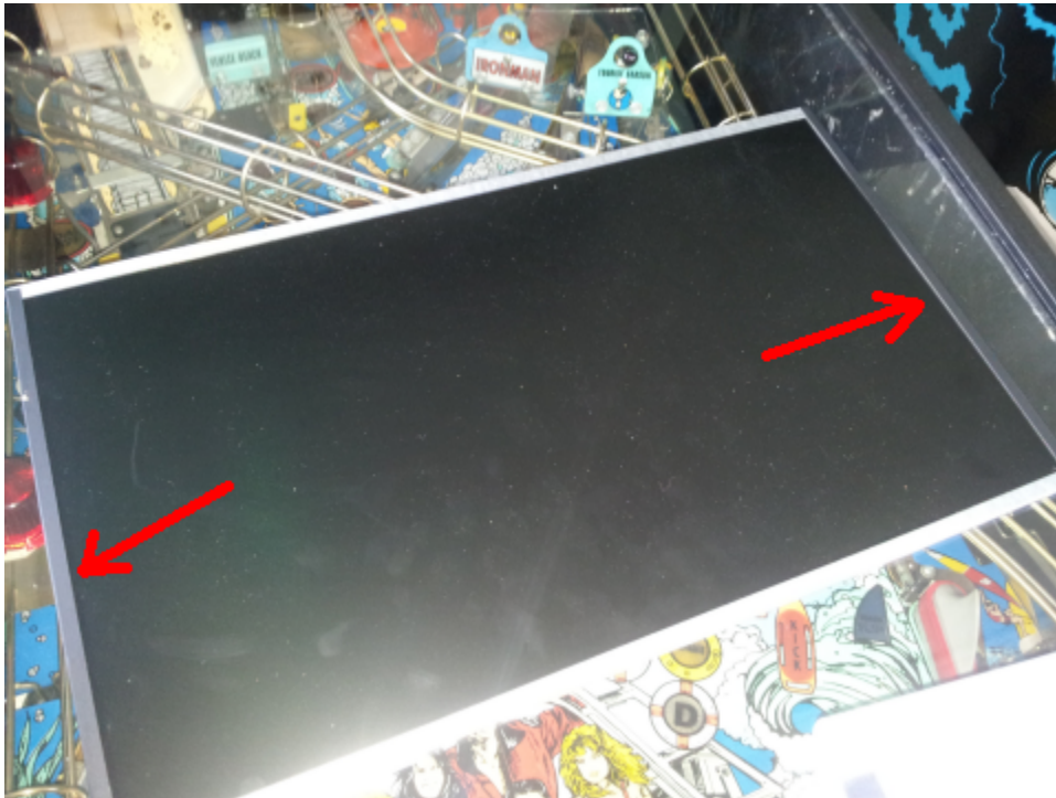
Figure 14 – Black insulation tape on left and right sides of the LCD panel
