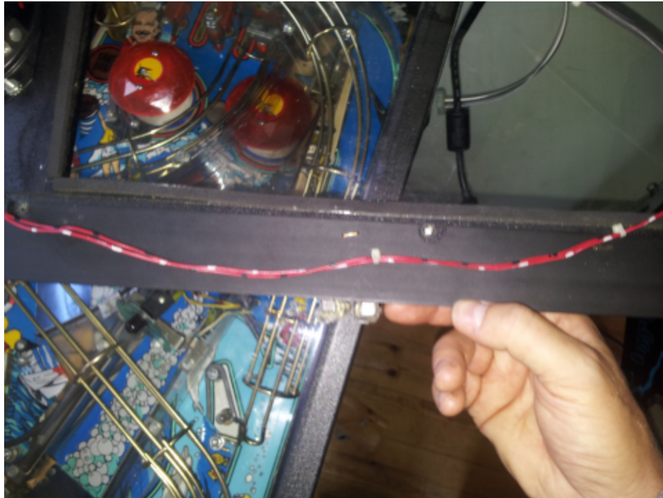
Figure 9 – Locate the staple over the side rail when using the hammer
