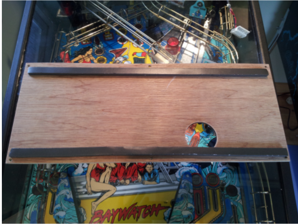
Figure 11 – Foam weather strip on the back of the plywood mounting plate
